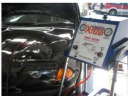
Power steer flush machine in action on a vehicle
