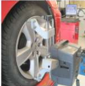
A sensor attached to the rim of a front wheel. The base computer unit is in the background with a graphic image on the screen showing the current alignment settings for this vehicle.
