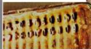
Rust & scale deposits on a radiator, blocking water jackets & restricting anti-freeze circulation.
